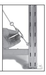
Insert another cross brace clip into a corresponding slot diagonally opposite and hook on the other end of the cross brace wire. Tighten the tensioner until the wire is taught. Repeat for the opposite side ensuring both tensioners are equal
