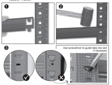
2. Assemble end frames with short side beams & join with long front & back beams
