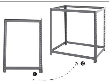
**3.** Bend centre support ends at right angles. Slot into front & back beams.
