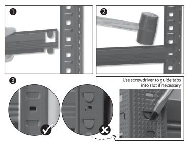
2. Assemble end frames with short beams & join with long front & back beams
