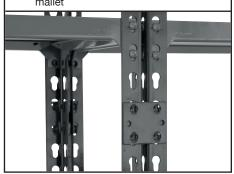
For tall or narrow shelving we recommend wall fixing where possible. Use Wall Ties towards the top of each bay and fix with suitable screws and plugs (not provided)
