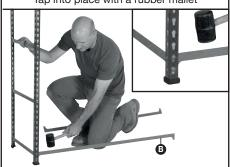
Insert the other ends of the beams Into the second frame as in step 5
