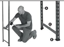
Tap beam • with a rubber mallet to ensure the end studs are fully located in the bottom of the keyholes
