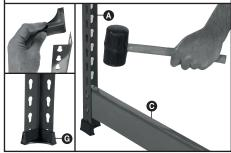
Tap beam with a rubber mallet to ensure the end studs are fully located in the bottom of the keyholes on both uprights. Lean the uprights against a wall for support if needed
