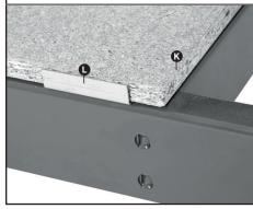
Add the 'L' section beam to the top of the rear uprights. This will support the back of the louvre panels which can be assembled on the worktop in front, as below. Join the panels together with 8x nuts and bolts supplied
