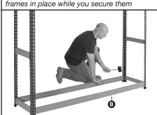
Repeat steps 5 and 6 to add the remaining long beams. Ensure that each long beam is located at the same height as the side beams
