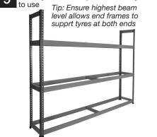
Tyre racks can be joined together with Tie Plates. Use 4 per join – 2 front and back. Knock into place with a rubber mallet
