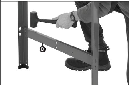
**8** Insert drawer support beam **E** into keyhole at the top of the uprights, leaving two keyholes clear at top. Knock beam into place with a rubber mallet
