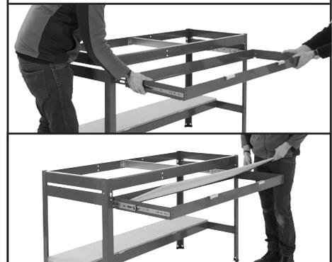
**22** Place chipboard deck **M** onto the top beams and locate using the uprights as a guide
