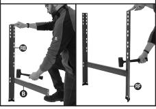
Slot drawer support beam (1) into the uprights. Leave two keyholes clear at top. Knock beam into place with a rubber mallet.
