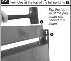
Add cantilever top shelf beam 1 to the other two keyholes at the top of the tall uprights A. Knock into place with a rubber mallet.
