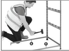
7 Insert the other ends of the beams of the beams into the second frame as in step 6 Tip: Ask another person to hold the frames in place while you secure them
