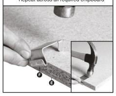
12 Insert chipboard panels into shelf beams ensuring they sit onto the top ledges and the clamps hook over the edges as below
