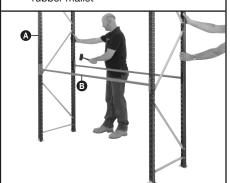
Insert safety clips **②** into the holes at each end of the rails **③** to ensure the rails cannot be removed from the upright
