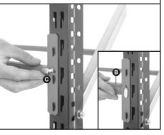
8 To extend the shelving, add support beams (a) to the second frame (a) and repeat steps 1 to 5 to add extra beams
