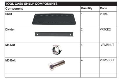
1 Position shelf to required height remembering that shelf sits one tab higher on the front than the back with the folded lip on the back
