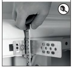
8 Slide the racking unit(s) against the side wall & fix to the brackets (you may need to drill suitable holes in the van racking frame to match the two.
