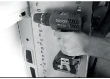
6 Cut out holes in the ply lining so that the brackets fit through
