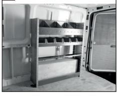
5 Fit the ply lining against the side of the vehicle and carefully measure the bracket positions
