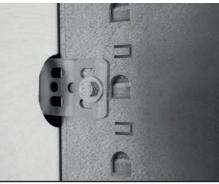
3 Mark Bracket locations and drill holes into the double seam making sure when drilling not to go through the outer skin of the vehicle
